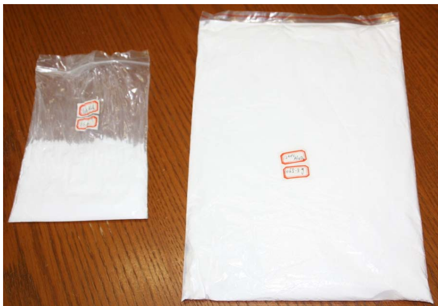
Figure 1: The samples of 99.99% high purity alumina (left) and 99% metallurgical grade alumina (right).
